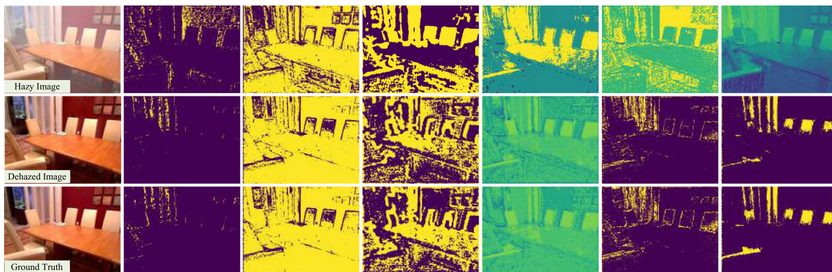
Fig. 4. Exhibition of multi-channel feature maps after using the PCFA module. The first row depicts the input hazy image and its six typical channels selected from the multi-channel feature maps handled by PCFA. The same six channels of feature maps generated from the dehazed image and corresponding ground truth are presented in the second and third rows, respectively.
